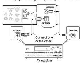
If your AV receiver doesn't support Dolby Digital and DTS, set the Digital/HDMI Audio Out setting to PCM. See page 48, and also refer to the operating instructions that came with your AV receiver.
